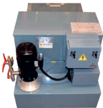
Effluent filtering system
